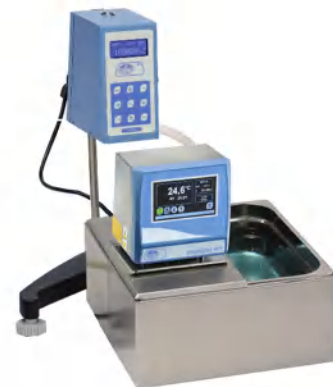
Immersion thermostat Digiterm controlling temperature of viscometer.
